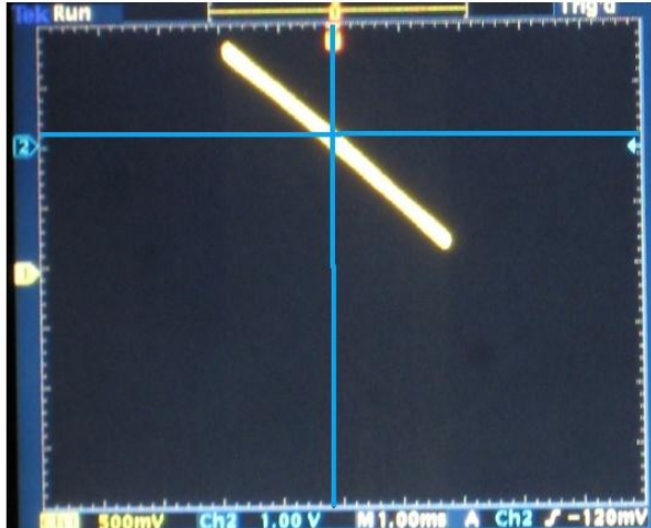
From [3], pinched-hysteresis for 35 kHz sinusoidal input
