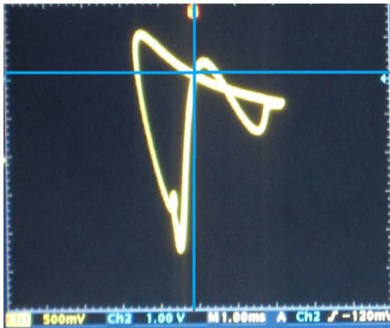
From [3], pinched-hysteresis for 3 kHz sinusoidal input
