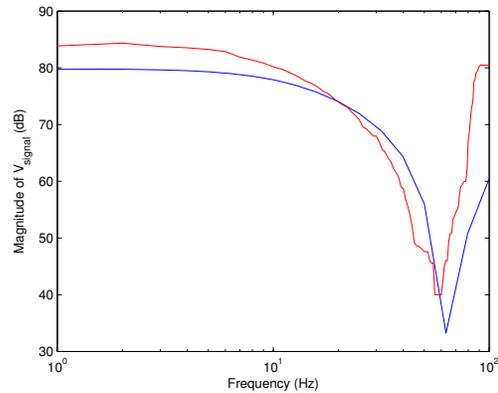
Fig. 3: The simulation bode plot (blue) versus the experimental bode plot (red). Simulation was carried out using MultiSim [8] (a SPICE [10] graphical front end). Experimental data was obtained by using a 80 dB attenuator to input a 100  $\mu\text{V}$  sinusoid with varying frequency and then measuring the amplitude of the output.
