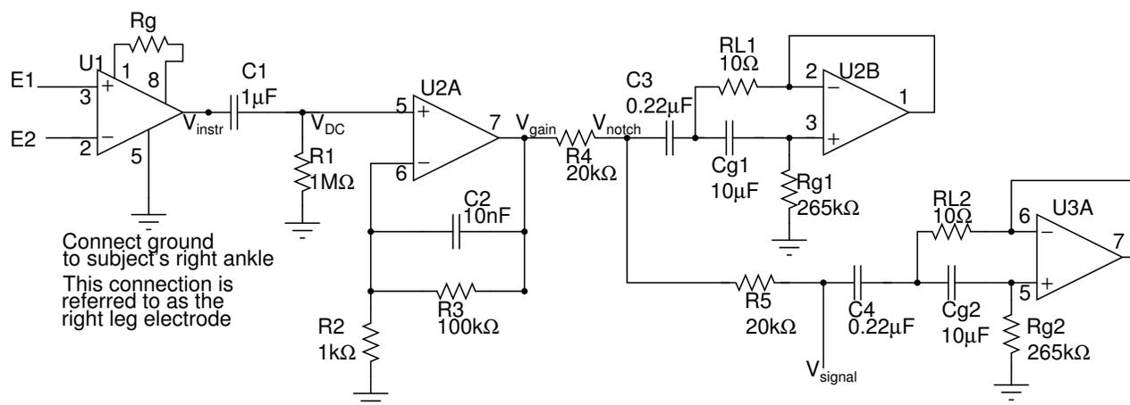
Fig. 1: The analog subcircuits for the mixed-signal EEG interface. The instrumentation amplifier U1 is an INA114, the operational amplifiers U2 and U3 are TLC277s. Since a discussion of transfer functions are included in first year electronics courses, the student is asked to derive theoretical transfer functions for the associated analog subsystems. For clarity purposes, the power supplies and isolation circuits are not shown.
