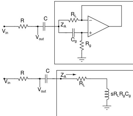
Fig. 2: An RCL notch filter. The inductor is realized using an operational amplifier based gyrator or impedance inverter.
